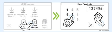
The oven downloads the recipes onto the USB drive. The default name for the file generated is ui\_dump.ai2. If another file with the same name is present, the oven will add numbers after the name so that no file is overwritten: ui\_dump1.ai2, ui\_dump2.ai2, ui\_dump3.ai2 and so on.
