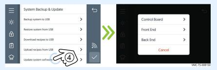
**Touch** Control Board (CB) to update the control board. The oven loads the selected software. The oven verifies the file and then updates the CB.
