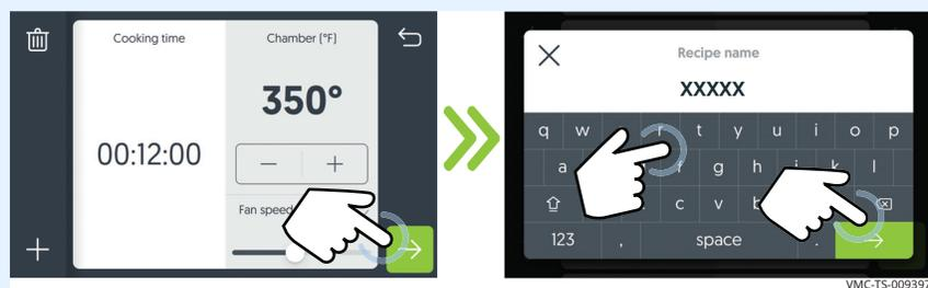
Step through the remaining screens using the forward arrow icon. Change the parameters of the recipe as desired. When you get back to the **browse recipes** screen, the changes will be saved and the recipe will be visible on the display.
