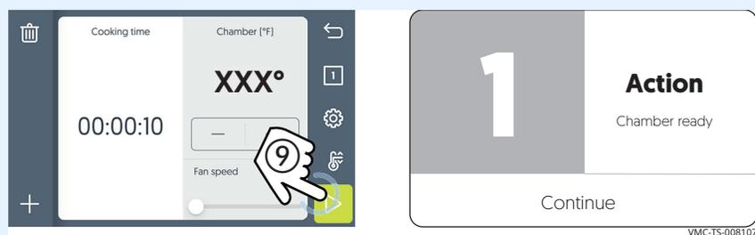
At the end of the preheat stage, the oven sounds an alert, and both the chamber light and the door handle light flash.
