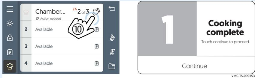
At the end of the cooking stage, the oven sounds an alert, and the chamber light and door handle light flash.
