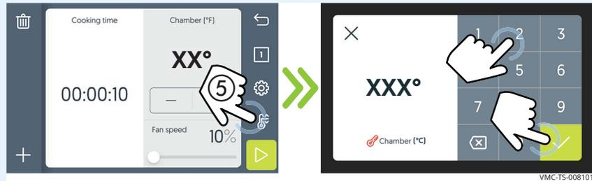
4. Now set the cooking parameters. **Touch** the cooking temperature ⑥. **Enter** the cooking temperature using the key pad.
