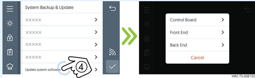
**Touch** Control Board (CB) to update the control board. The oven loads the selected software. The oven verifies the file and then updates the CB.
