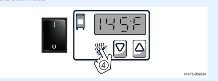
8. Allow the drawer warmer to re-stabilize and **compare** the temperature again. Tolerance at  $140^{\circ}F$  ( $60^{\circ}C$ ) is +/-  $8^{\circ}F$  (+/- $4^{\circ}C$ ). Tolerance at  $180^{\circ}F$  ( $82^{\circ}C$ ) is +/-  $10^{\circ}F$  (+/-  $6^{\circ}C$ ).
