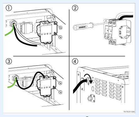
$\textbf{Re-install} \text{ the circuit breakers with the screws } \ensuremath{\mathfrak{G}}.$
