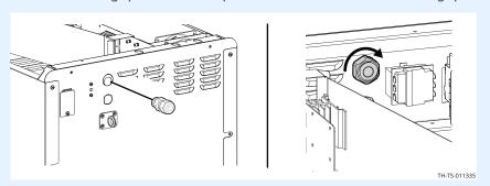
3. **Install** the cord through the cord grip. **Route** the ground wire to the terminal block.
