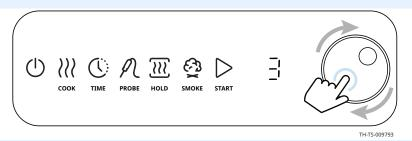
5. On double cavity ovens only, **turn** the knob to select the cavity to save the recipe to (top, bottom, or both).
