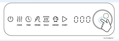
3. **Turn** the knob until the control displays USB.
